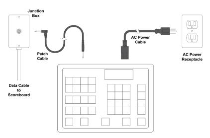
If your scoreboard package includes a ScoreLink RF Communications system, the power receptacle may be the only consideration on the control console side of the installation process. For details about ScoreLink, consult the documentation that ships with the product. Otherwise, use the stereo patch cable to plug the console into the junction box.
